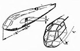
Fig. 1.—The carved fuselage block and (" A ") the framework of the nose cabin
