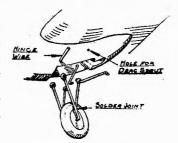
Fig. 3. — The main component parts of a simple form of retractable undercarriage
